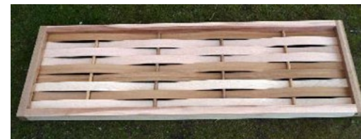
Timber connection inspired by bulrush mats
